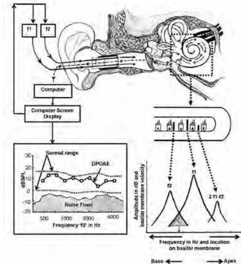
**Figure 2.** Illustration of the measurement of distortion product otoacoustic emissions (DPOAEs) showing a probe assembly that fits into the external ear canal, the delivery of the signals to the ear via the middle ear, the generation of OAEs by outer hair cells in the cochlea and, finally, propagation of OAE energy as sound into the external ear canal. Illustration appears with permission of artist Anuradha Bantwal.
